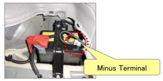
2.Remove the "Service Plug" of the main battery. (Caution) Electricity remains in inverter.
