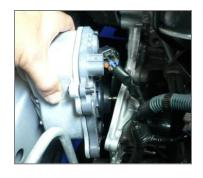
7.Install the new water pump, insert the connector until click, and install the air cleaner.
